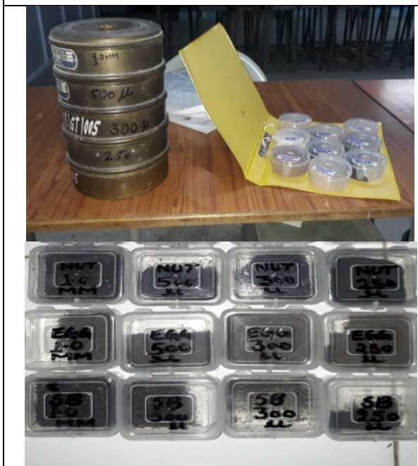
Fig.5: Sieve analysis using sieves of 250µm, 300µm, 500µm and 1.0mm sizes respectively.
